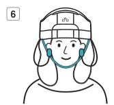
Attach the sensors to each earlobe for the measurement then adjust the chin strap.
